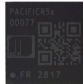
BGA package 12 × 12mm 2 196pins
