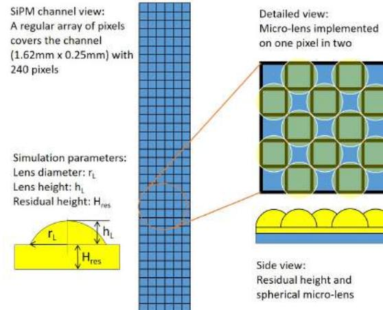
Better SiPMs and micro-lensing should compensate for light loss
