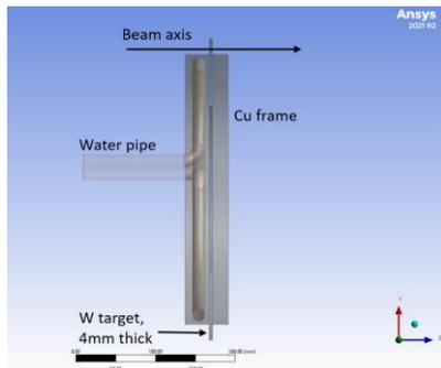
120 kW  $e^-$  beam irradiates water cooled spinning tungsten target,
