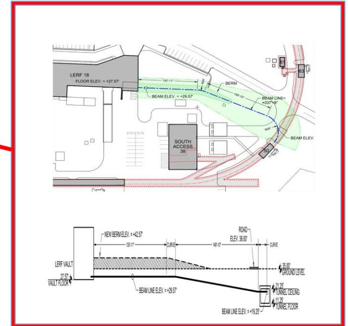
$e^+$  transported in new beamline and injected to CEBAF for 12 GeV, with magnet polarities reversed
