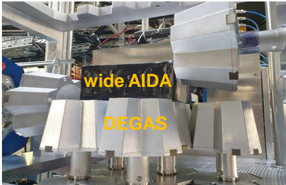
DESPEC High-resolution set-up with novel DEGAS Ge detectors
