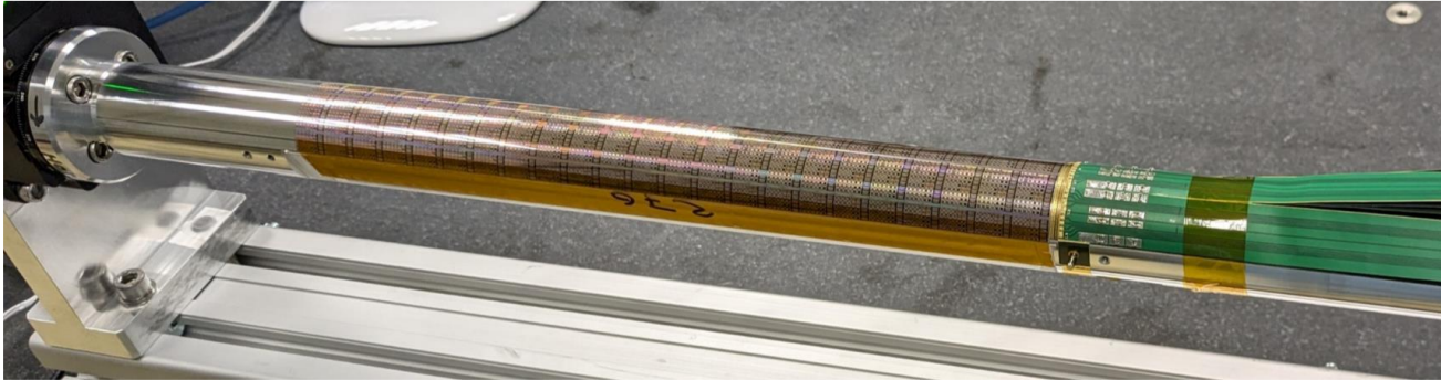
FPC and Sensor on jig
