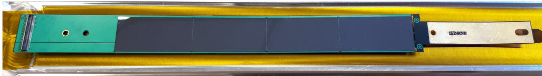
Alice MFT 4 chip ladder, https://cds.cern.ch/record/2748315
