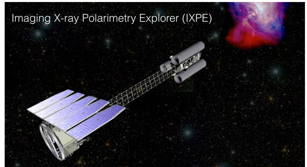
The Imaging X-Ray Polarimetry Explorer (IXPE) is an X-ray telescope capable of extracting information on the X-ray polarization of astrophysical sources in the 2-8 keV band. After a successful launch, IXPE started science operations in January 11 2022.
