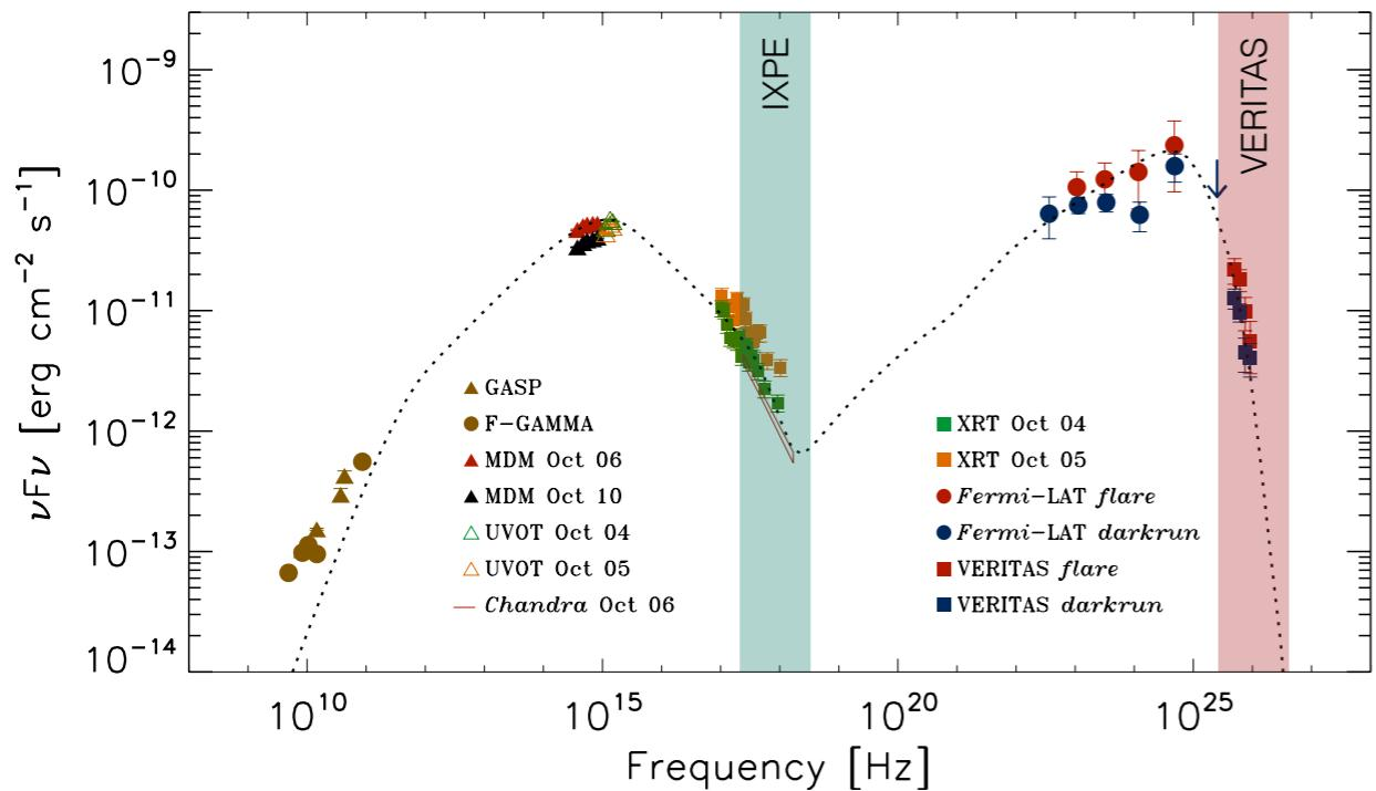
SED of 3C 66A (Abdo et al. 2013). The energy coverage of IXPE and VERITAS probes the same part of the emitting particle spectrum.
