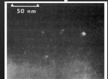
Fig. 1 Dark-field transmission electron micrograph of Allende CJ, in which bright areas are diamond grains diffracting electrons into one part of the innermost ring of the diffraction pattern shown in Fig. 2. As most grains do not have the proper orientation, the true abundance of diamond is perhaps five times higher than indicated by the bright areas in the picture.
