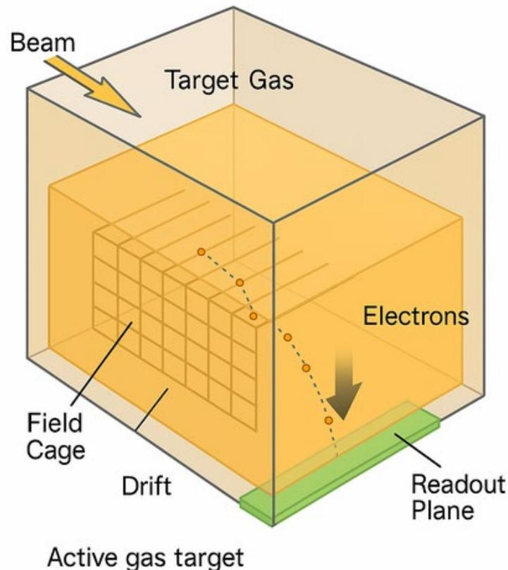
**Functioning principle:** It is all about **ionization** & **drift**
