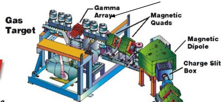
Primary beam rejected (E and B fields set to transport recoils and stop primary beam on slits)
