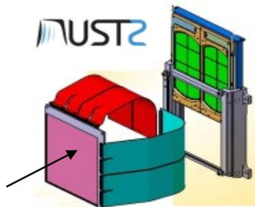
First layer: **DSSD** (double sided strip detector) (300 μm, 128 strips in X & Y)
