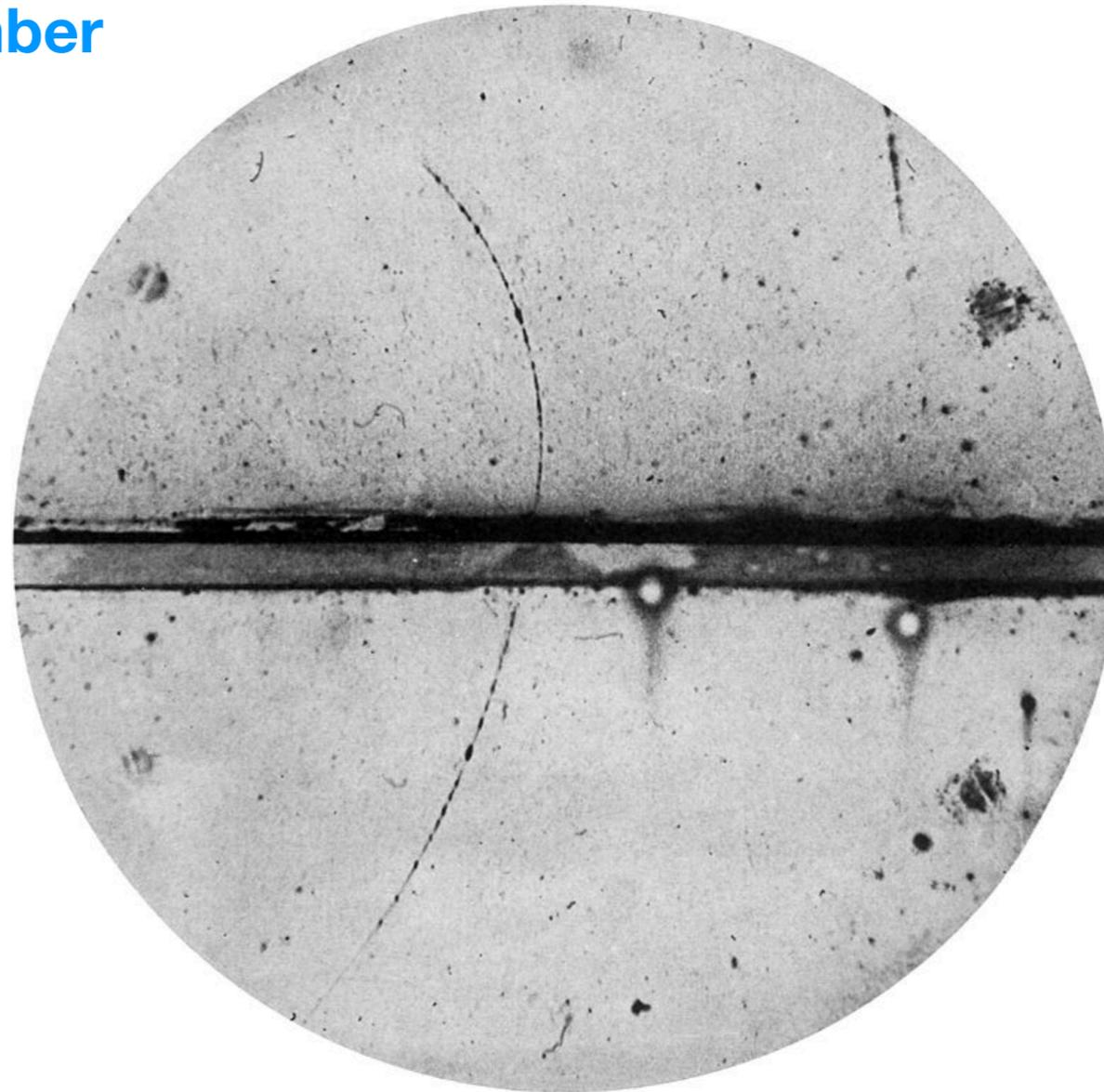
Cloud chamber track of the **positron**, discovered by **Carl Anderson in 1932**. The positron was predicted by **Paul Dirac**. Anderson discovered it in CRs for the first time, whereas later experiments with gamma-rays produced in radioactive nuclei resulted in the creation of positron-electron pairs. For this work Anderson shared the Nobel Prize in Physics in 1936.
