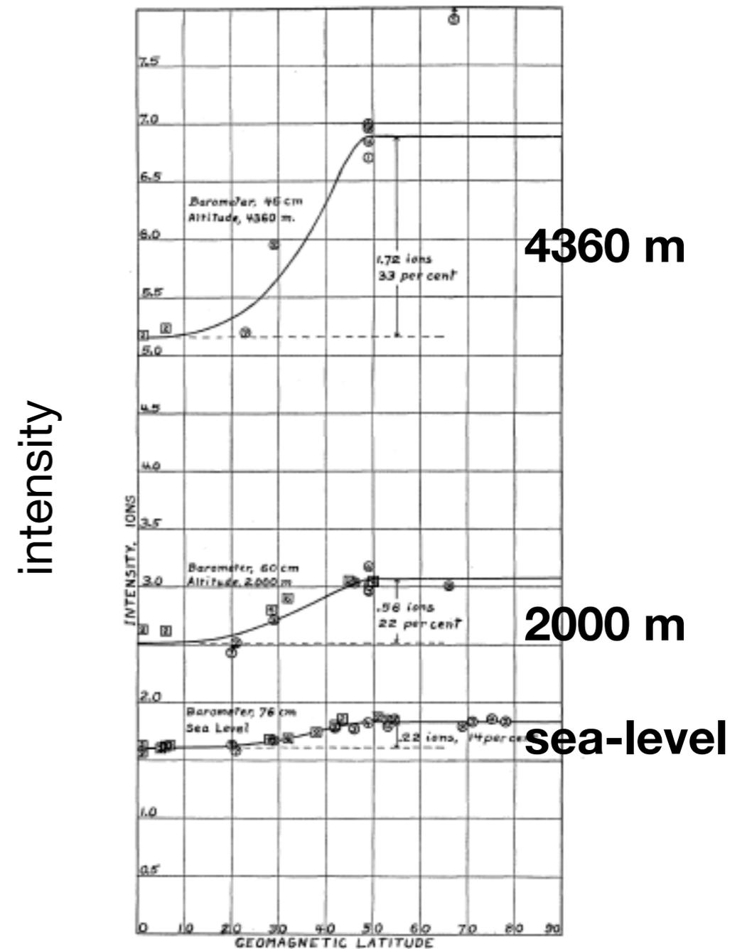
FIG. 6. Intensity vs. geomagnetic latitude for different altitudes
