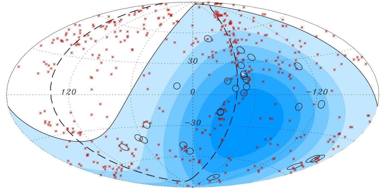
**Arrival directions of UHECRs measured with Pierre Auger Obs. For  $E > 57 \times 10^{18}$  eV,  $D_{\max} = 75$  Mpc,  $\Psi = 3.1^\circ$ , 8 out of 13 events correlate with AGN locations, implying  $P < 1.7 \times 10^{-3}$  for these to occur by chance if flux is isotropic**
