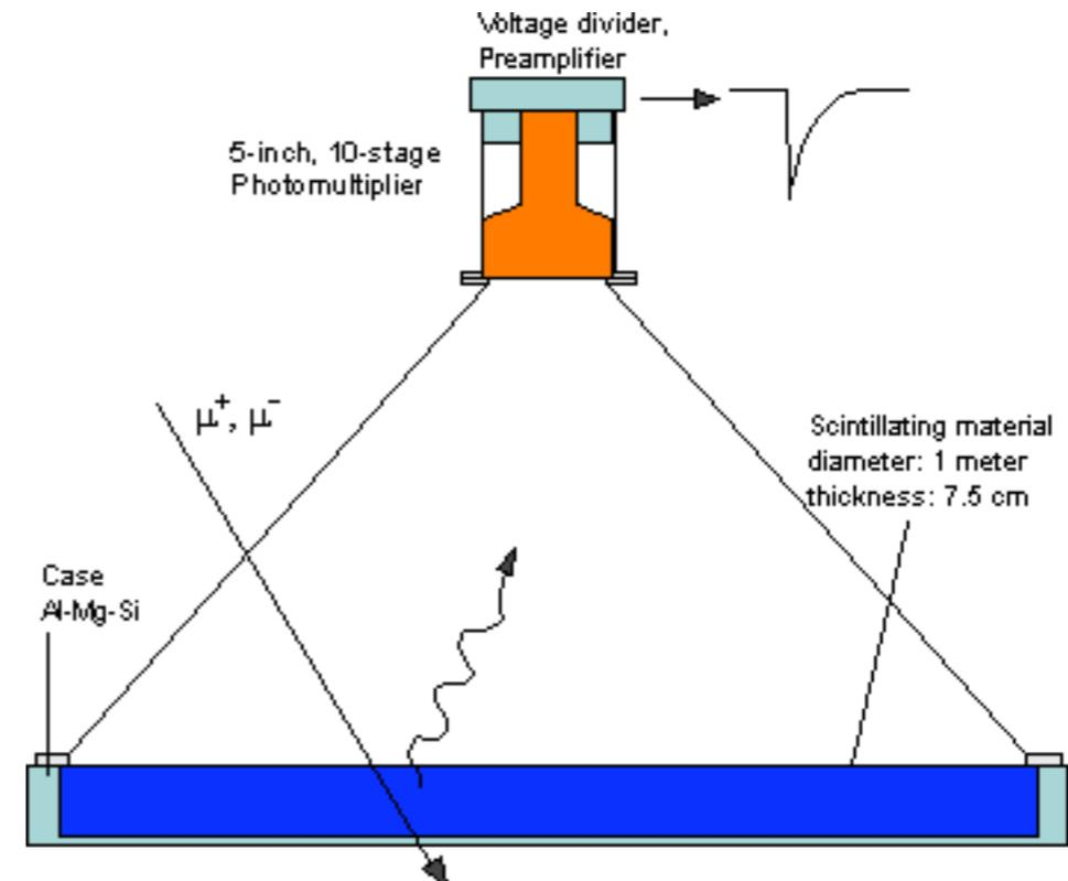
*scheme of a scintillator coupled to a PMT*
