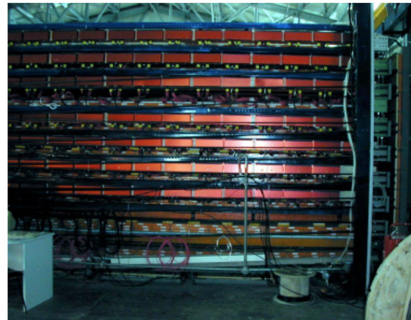
**calorimeters for muons and hadrons**
