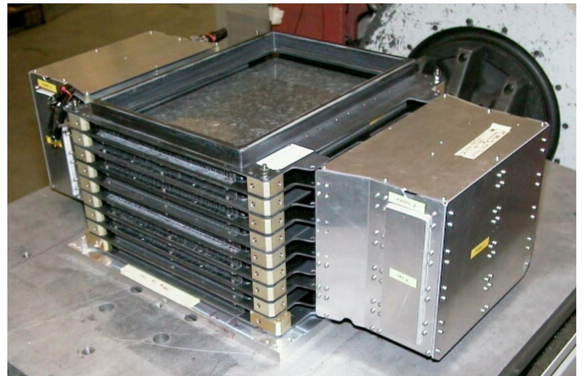
*the transition-radiation detector of the PAMELA experiment*
