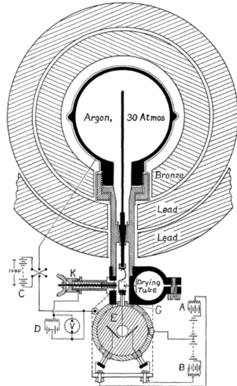
FIG. 2. Cosmic-ray ionization chamber, electrometer, and electrical connections
