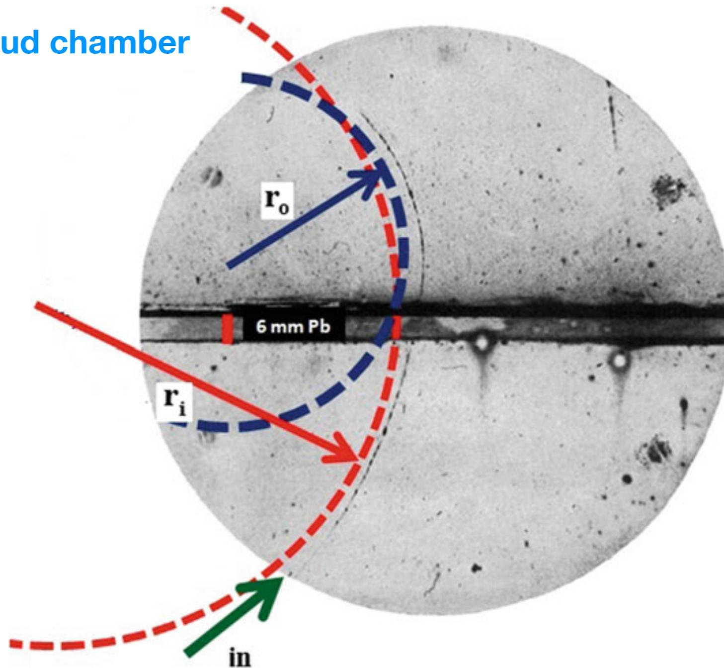
Cloud chamber track of the **positron**, discovered by **Carl Anderson in 1932**. The positron was predicted by **Paul Dirac**. Anderson discovered it in CRs for the first time, whereas later experiments with gamma-rays produced in radioactive nuclei resulted in the creation of positron-electron pairs. For this work Anderson shared the Nobel Prize in Physics in 1936.
