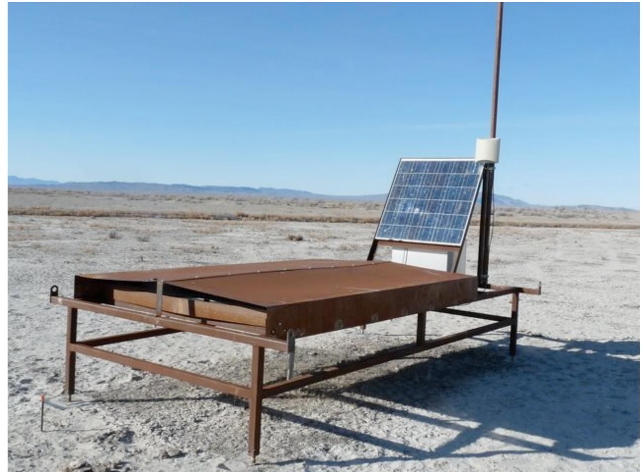
*a plastic scintillator in the Utah desert from the Telescope Array experiment*
